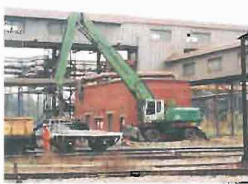
Transportation – EXCAVATOR WITH SENNEBOGEN MAGNET 840M 20T
